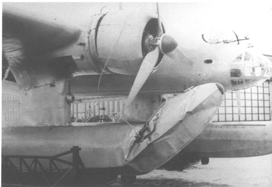
Ha 140 V1 coded D-AUTO suffered an accident in December 1937; this photo shows the damage to the starboard float and engine which occurred when the aircraft landed in rough seas.
