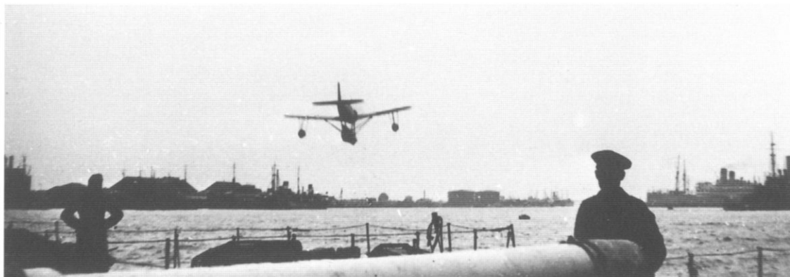
A second series Ar 196 prototype, either V3 (Wk Nr 2591, D-ILRE), V4 (Wk Nr 2592, D-OVMB), or V5 (Wk Nr 0090, D-IPOB). The main difference from earlier and later Ar 196s was the float arrangement. (Drogen-Meyer, Wilhelmshaven)
