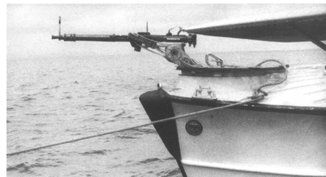
A Dornier Wal with an experimental 20mm cannon fitted in the nose. (Griehl)
